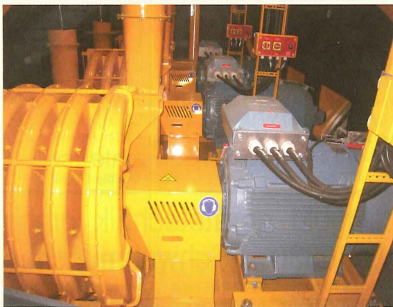
Fig. 3: Three turbo blower groups provide the air flow to unload 500 tonnes of wood pellets per hour.
