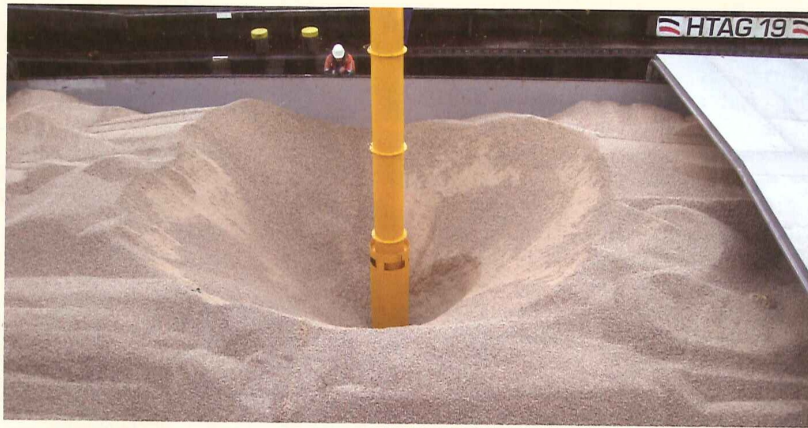
Fig. 2: Pneumatic unloading of wood pellets prevents any dust from being raised.
